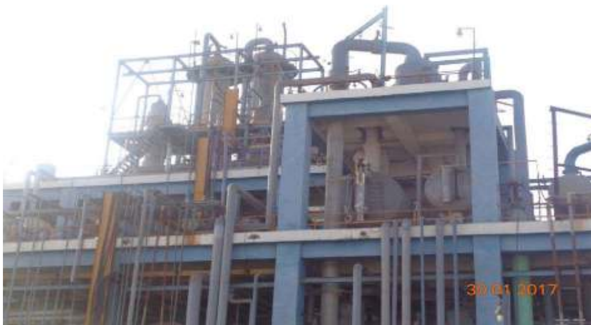
Scrubbing System for HCl generated from Chloromethane
